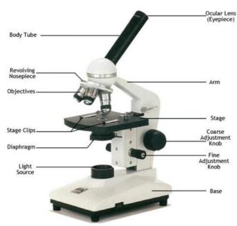
Table 10.2 The parts of a compound light microscope
